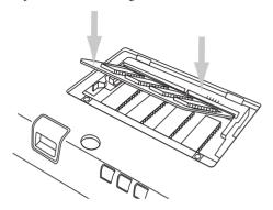
Figure 2-8. Installing a DIMM Module
